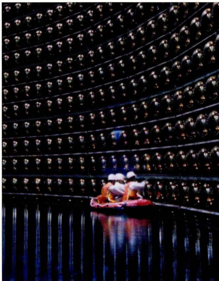
One of the clients of the new Japanese proton facility would be the Superkamiokande underground neutrino experiment, 300 km from the Tokai site. Here, researchers are carefully cleaning the photodetectors as the neutrino target volume is filled with water.
