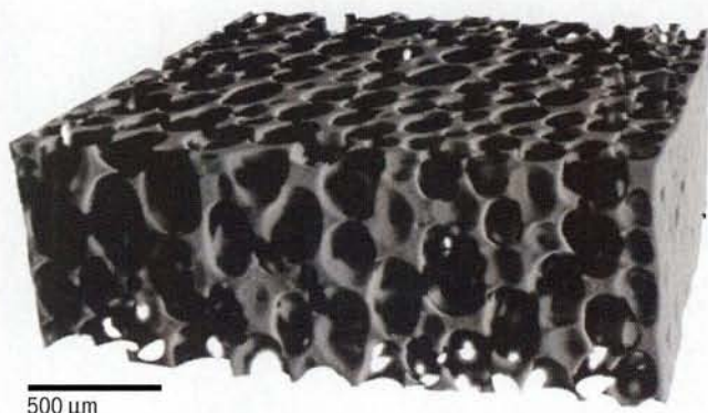
Industrial foam viewed by X-ray microtomography using coherent light from a third-generation synchrotron. (ESRF.)
